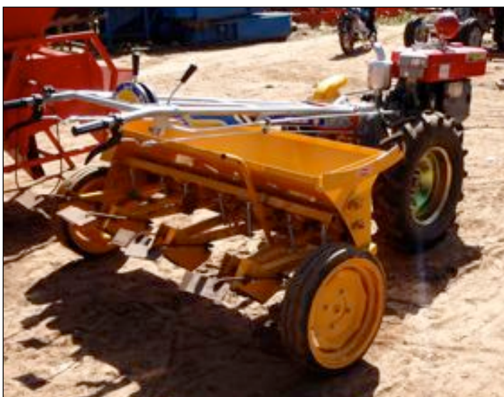
Prototype seeding machine developed by CAFON, attached to a hand tractor.
